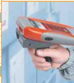
For the frequent scanning, Pistol Grip provides more ergonomics and safe handling of the Communicator.
